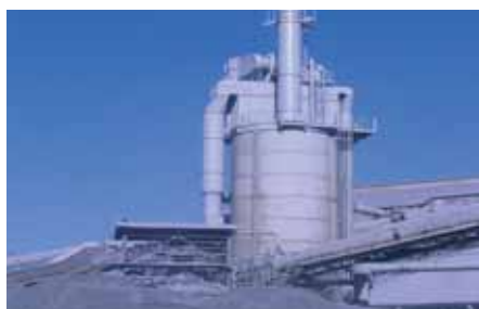
Dust collectors for mineral treatment, e.g. on jaw and rotary crushers, impact crushers, screening machines, conveyor belts, air separators, silo aspirators and loading stations.
