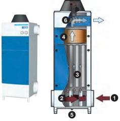
The filters in the NOM series are intended for machines that punch and press steel sheet, for industrial washing machines, for abrasive water-cooled cutting, etc. In all metal fabrication processes where there are problems with oil mist, these filters can be mounted in a pipework system connected to the machines.
