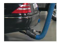
Nederman offer an extensive range of robust rubber and metal nozzles to accommodate various types of vehicles and systems. Adjustable test funnels with special design to handle large volumes of hot exhaust from vehicles in inspection centres for example.
