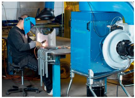
Complete mobile FilterBox unit with Original extraction arm.
