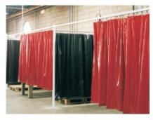
Standard sized curtains (see below) provided with 50 mm welded seam all around and with snap-fasteners on both sides for joining to obtain total desired width. Supplied with reinforced holes in the upper edge and steel suspension rings. All standard curtains are made of pliable self extinguishing PVC material with flash point 320-390°C.
