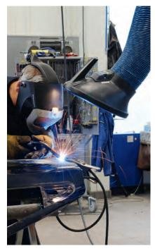
It is specially designed for working environments with fumes, vapours or non-explosive dust. Typical workplaces are the metal fabrication industry or other types of industries where extraction is needed. The applications can be welding, grinding, or other industrial processes where an easily positioned arm is required. The product is equipped with a damper in the hood as standard.
