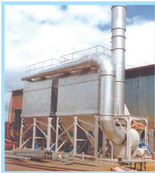
Fume extraction from hot-dip galvanizing process
