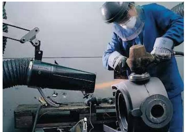
*Grinding particles are safely collected by an extraction and filtration system*
