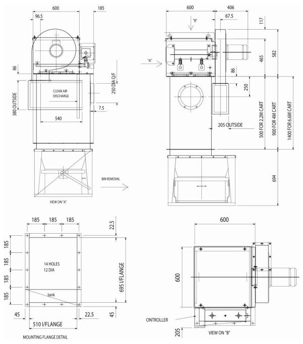
The MJC Mini 9/22/22, 16/40/22 and 26/66/22 are available as insertable or open based venting filters, with or without fan assistance. Both units use the same mounting flange illustrated here.
