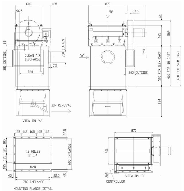
The MJC Mini 13/22/32, 24/40/32 and 40/66/32 are available as insertable or open based venting filters, with or without fan assistance. Both units use the same mounting flange illustrated here.
