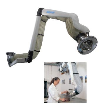
The Nederman DX has a double earthed system, antistatic earthed ventilation hose that prevents static electricity and sparks. The arm is suitable for industries where hygiene is a top priority. NEX DX has concealed joints and a separate easy to mount hose. Enclosed support arm, separate hose and a stainless steel hood means the DX arms require little maintenance and is easy to clean.
