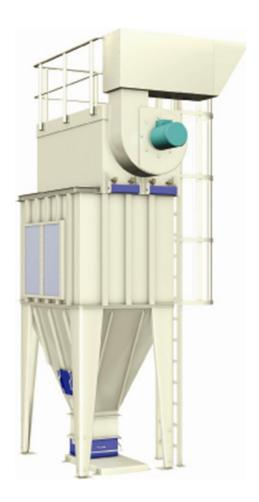
The MJC is a long established range of reverse jet cleaned tubular cartridge filters designed for continuous operation in process and general dust extraction applications with free flowing dust. This recently upgraded filter range offers two filter cartridge lengths and on-line high efficiency reverse jet cleaning. Filter areas range from 48m² to 739m² as standard, utilising patented UniClean cartridges. However, units up to about 1050m² may be made to special order.
